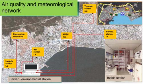
u.s – *urban station* t.s – *traffic station* m.s – *meteorological station*  The following Table presents the monitored pollutants in each station of the network. Meteorological data (wind speed, wind direction, temperature, relative humidity) are recorded in all stations except for Agia Sofia and Pl. Dimokratias stations.
