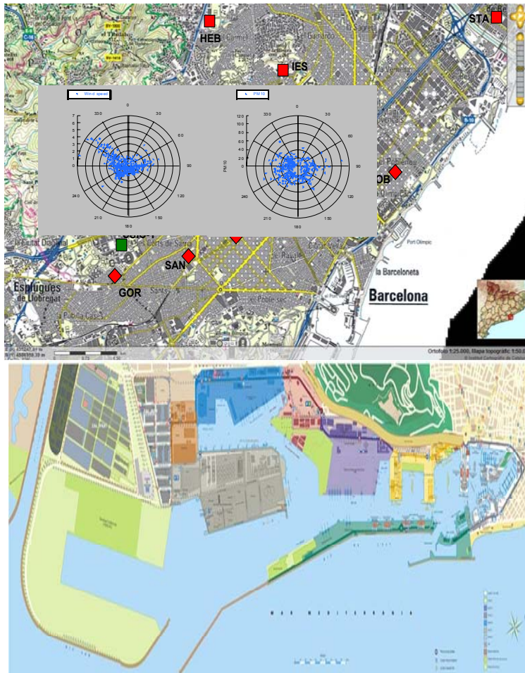
Fig.20 PM10 concentration rose ( \mu\text{g}/\text{m}^3 , degrees) and wind speed rose (m/s, degrees) for the year 2009-activities in Barcelona.
