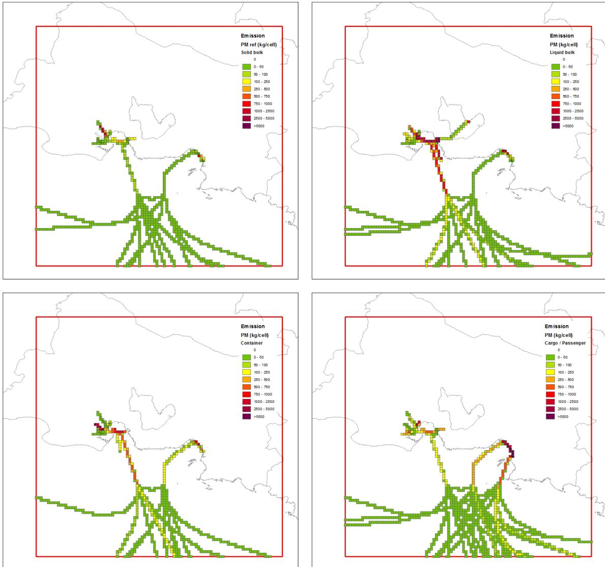
Figure 6: Total annual PM<sub>2.5</sub> emission (on-route, maneuvering and hotelling) for solid bulk, liquid bulk, container and cargo/passenger over the APICE domain (reference year 2007).
