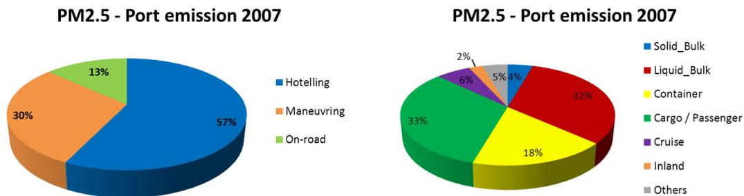
Figure 5 : Contribution of different phases and different activities for the total emission in Marseille port for PM2.5 (reference year of 2007).
