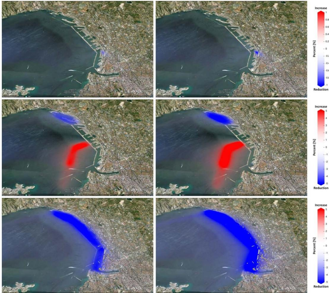
**Figure 6:** Relative difference between the “Base future” and the “Cold ironing” scenario (top), the “New cruise terminal” scenario (middle) and the “LNG passenger” scenario (bottom) for the PM10 (left) and PM2.5 (right) concentrations during the winter period over the urban domain for Marseille.
